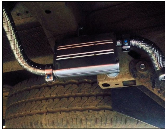
Fig 11 – The exhaust or combustion pipe must be located so that they cannot be clogged by dirt or road debris
