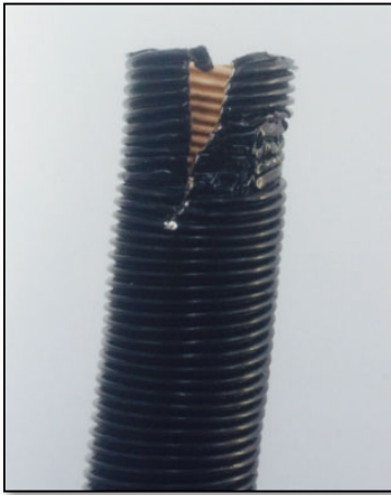
Fig 9 – Combustion Air Tube “V” cut.
