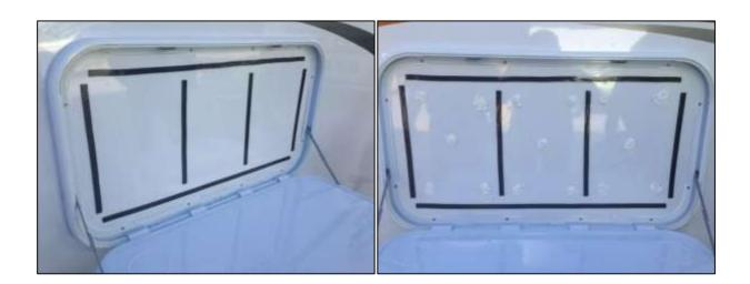
**Step 10:** You are now ready to install the backing plate. Simply align the edges of the backing plate with the internal frame and gently push into position. Please take care in this step as once the double sided tape has adhered, it will be difficult to remove the backing plate to have a second attempt.
