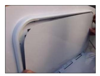
**Step 11:** If required, apply a bead of appropriate silicone/sealant all around the edge of the picnic table to give it an aesthetically pleasing finish.
